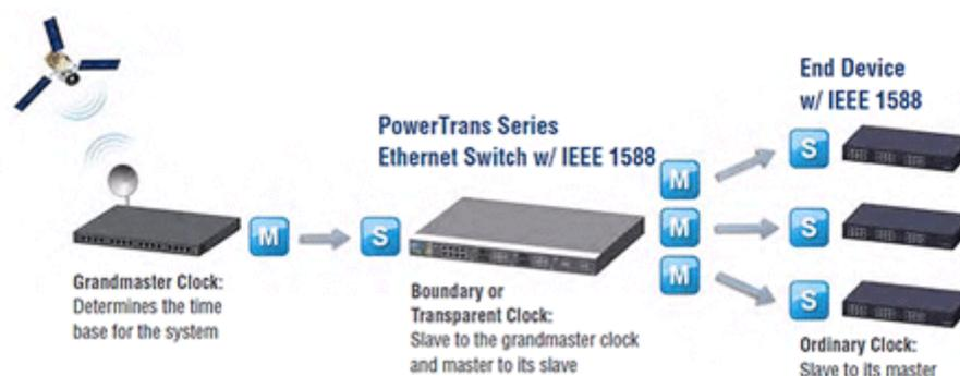
*An IEEE 1588v2 system needs just one GPS receiver to provide highly accurate time information to many devices*
