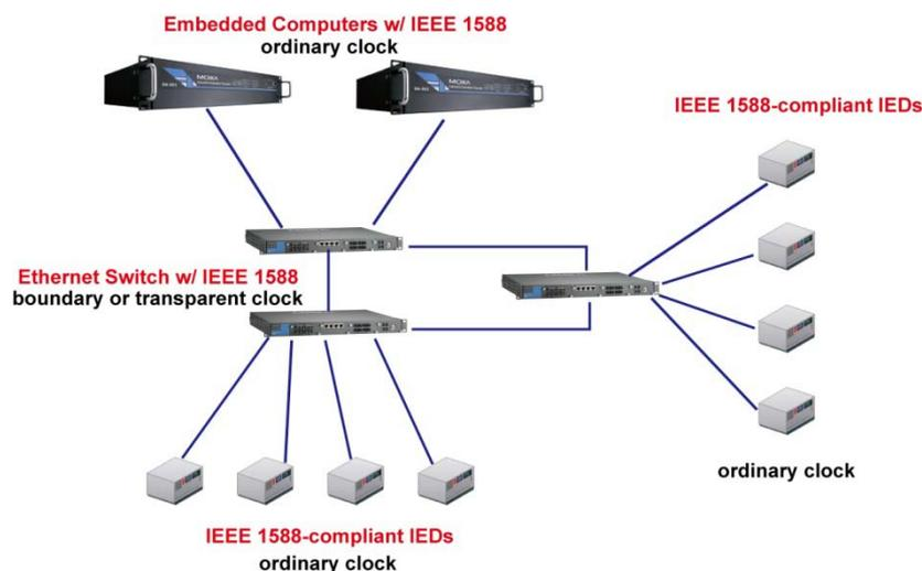
*To be in sync all of the system components, including the embedded computers, should support IEEE 1588v2*
